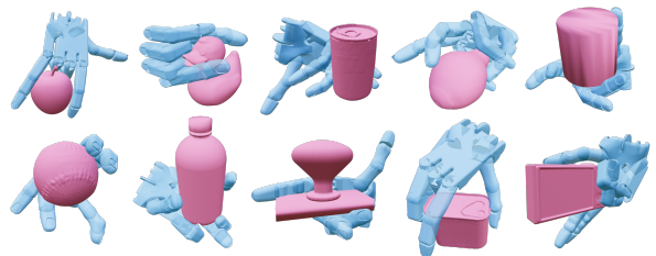
Fig. 11: Grasp examples filtered out from the dataset that would otherwise be deemed successful under static metric.
