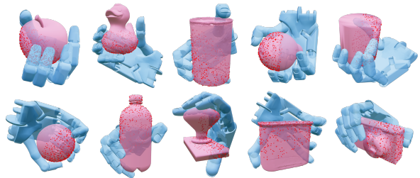
Fig. 9: Grasp examples with partial object point clouds. Red points show the observed portion.
