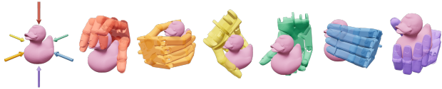
Fig. 5: Diverse and pose-controllable grasp generation. The arrow refers to the input palm orientation. Arrows and hands of the same color represent corresponding input-output pairs.
