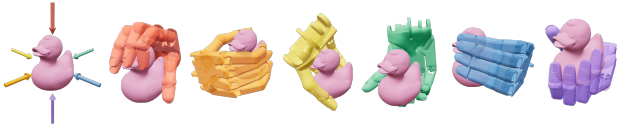
Fig. 5: Diverse and pose-controllable grasp generation. The arrow refers to the input palm orientation. Arrows and hands of the same color represent corresponding input-output pairs.
