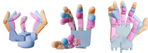
Fig. 10: Visualization of the grasp controller's effect: blue indicates the predicted grasp pose, orange represents q_{\text{outer}} , and pink represents q_{\text{inner}} .
